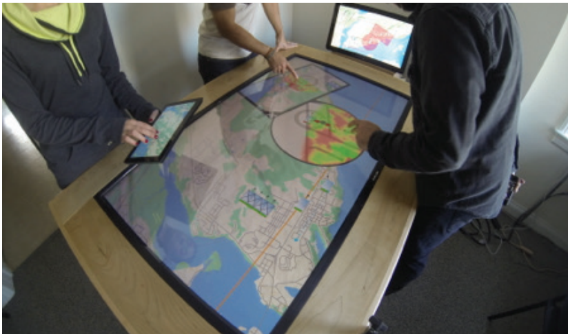
Figure 1. OrMiS supports military simulation by allowing small groups of people to collaborate around a shared touch surface. OrMiS is based on a large multi-touch table, handheld tablets, and a radar view display.
