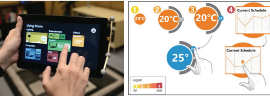
Figure 6. (Left) Proxemic-aware remote controls: remote control interface on a tablet computer; (Right) thermostat interface, showing a series of progressively revealed interaction controls on the remote control's screen (Ledo, Greenberg, Marquardt, Boring 2015).
